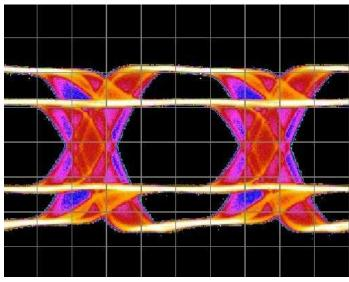
De-emphasized signal with sinusoidal jitter from a BERTScope.
